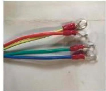
Instructions for connecting the motor (which has been left outside the control cabinet): the live wires are red, blue and green, the ground wire is yellow and placed where indicated by the arrow.
